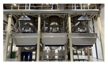
**Bottom discharge of distillers** – Post-distillation, spent seed material is discharged through bottom hatches into mobile containers. These containers are then transported to a separate district heating plant.
